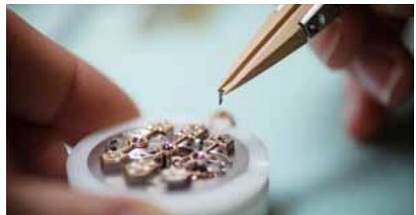
Assembly of the three gold Bridges on the movement
